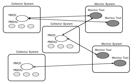
Figure 7.3. General PCP Deployment for Multiple Systems
