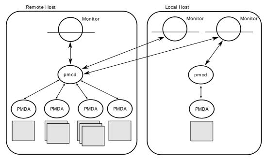
Figure 1.2. Process Structure for Distributed Operation
