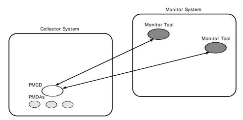
Figure 7.2. Basic PCP Deployment for Two Systems
